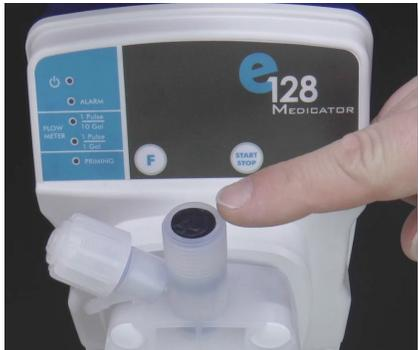
**Step 5:** Remove and discard the black shipping disc or transit washer, on the top of the discharge valve. You may need to use a flat blade screw driver to remove.
