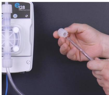
**Step 33:** Slide the open end of the PVC tubing through the outside opening of the tube nut.
