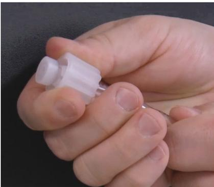
**Step 36:** Slide the tube nut toward the nozzle to compress the collar and nozzle tight together. This should form a ferrule connection.
