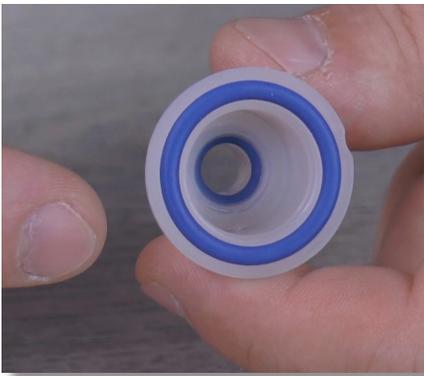
**Step 44:** While holding onto the ceramic ball, inspect the two blue o-rings in the grooves of the filter seat and make sure they are not damaged.
