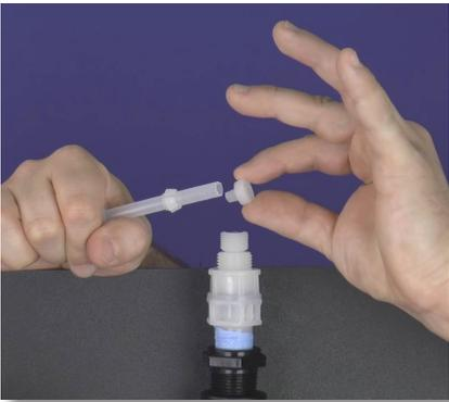
**Step 20:** Grab the nozzle and insert the pointed end into the opening of the same tube. Push the collar and nozzle together as close as possible.
