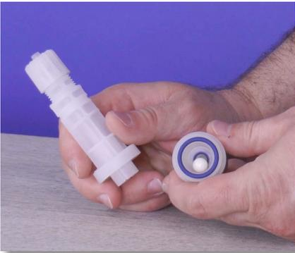
**Step 40:** Set the filter body aside and locate the ceramic ball in the filter seat.
