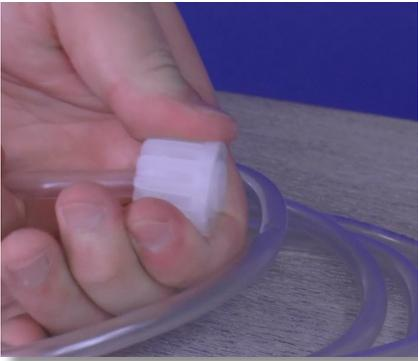
**Step 29:** Pull the tube nut toward the nozzle to compress the collar and nozzle tight together. This should form a ferrule connection.
