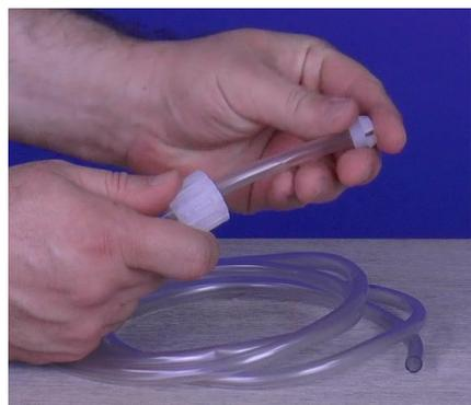
**Step 27:** Slide the collar onto the tube making sure the collar's crown is pointing away from the tube nut.
