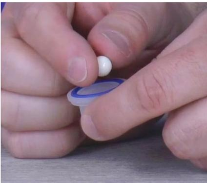
**Step 45:** Put the ceramic ball back into the filter seat and set the filter seat aside.
