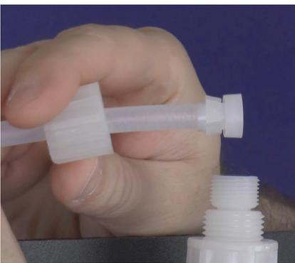
**Step 21:** Slide the tube nut toward the nozzle to compress the collar and nozzle tight together. This should form a ferrule connection.
