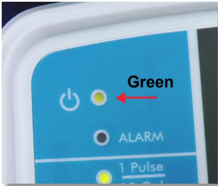
**Step 64:** Once again, press the **Start/Stop** button. The power LED will light up green and the **e128** is in **Stand-By Mode**, waiting for a signal from the water meter.
