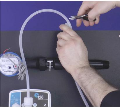
**Step 17:** Grab the rigid polyethylene discharge tube connected to the discharge valve. Using diagonal pliers, cut the tube so that it runs comfortably from the discharge valve to the injection valve.
