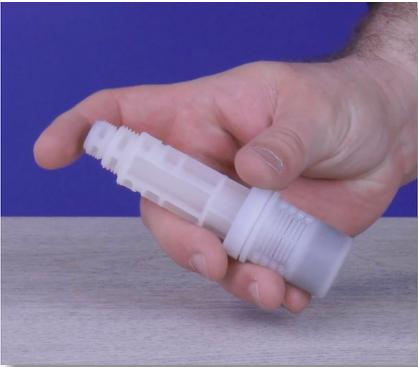
**Step 38:** Grab the foot filter and shake it back and forth. You should hear a ceramic ball moving freely inside.
