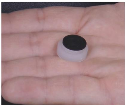
**Step 6:** If the black shipping disc or transit washer is not located on the top of the discharge valve, it may be stuck behind the nozzle, remove and discharge.
