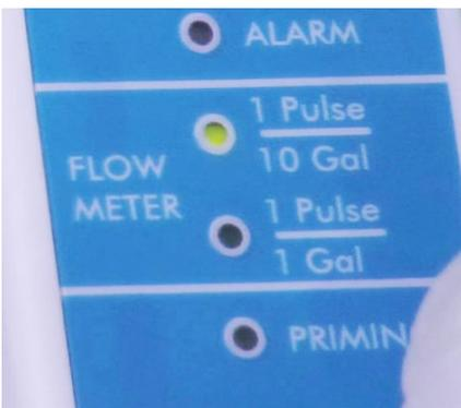
**Step 63:** Press the **"F"** button and select a program to match your water meter. Either 1 Pulse per 1 Gallon (1 GPC), or 1 Pulse per 10 Gallons (10 GPC).
