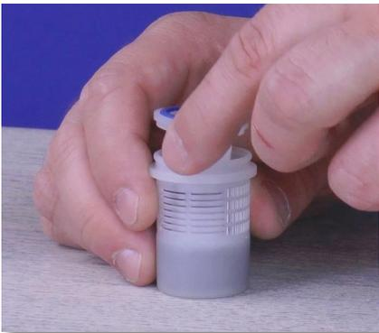
**Step 41:** Pull the filter seat out of the filter basket and set the filter basket aside.
