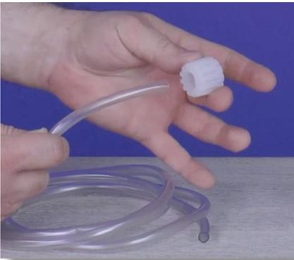
**Step 26:** Slide one end of the PVC tubing through the outside opening of the tube nut.
