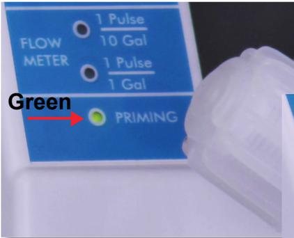
**Step 56:** Press the 'F' or function button a couple of times until the priming LED lights up green.
