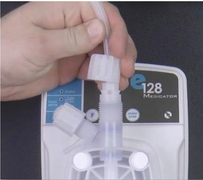
**Step 13:** Attach the tube, and tube connections onto the discharge valve by hand tightening the tube nut. Do not cross thread nor overtighten.
