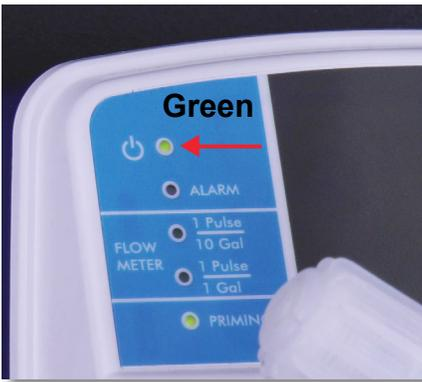
**Step 61:** When the priming process completes, the **e128 Medicator** stops stroking and the power LED lights up green. The pump is now in **Stand-By Mode**.
