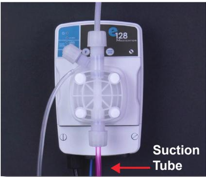
**Step 58:** The e128 should start stroking or clicking, and chemical should start coming up the suction tube.
