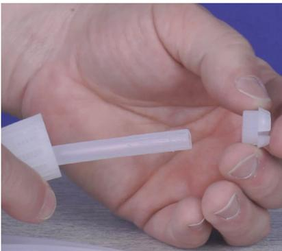
**Step 9:** Slide the collar onto the tube, and make sure the collar's crown is pointing away from the tube nut.
