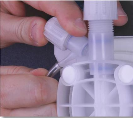
**Step 52:** Locate the manual air bleed barb on the upper left section of the pump's head and slide one end of the PVC tubing over the barb.
